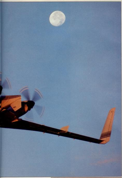
Want sizzle? Starship's got it—resin-bonded carbon-fiber structure, a pair of pusher turboprop engines, forward and main wings, and tip sails. There is no other shape like it at the flight levels. The leather-finished cabin is surprisingly conservative given the airplane's unconventional shape and technology. Baggage is loaded through the cabin and stowed aft of the rear seats.
