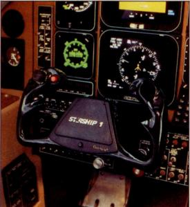
The Starship's futuristic image is reflected in the 16tube Collins instrument panel, designed expressly for the airplane. All navigation and communication information, including frequencies and identifiers, is fed to the black boxes via pilot and copilot keypads. Displays can be transferred among the various tubes. The only mechanical instruments are stand-by attitude and airspeed indicators and an altimeter.
